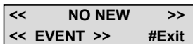
Fig. 3 - When all notifications have been displayed, the red LED turns off and the message in the figure is displayed
